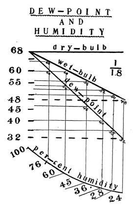
$70^{\circ}$ —the difference between the readings of the dry-bulb thermometer and the dew-point is always about 1.8 times the difference between the readings of the dry- and wet-bulb thermometers. The percentage of humidity, which corresponds approximately to these readings, is shown in the curved line below.
